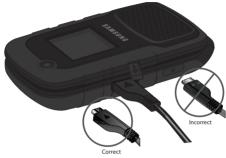
Note: The previous illustration displays the correct and incorrect method for connecting the charger. If the incorrect method is attempted, damage to the accessory port will occur therefore voiding the phone's warranty.
